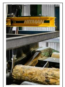
Hitman LG640-T tests logs on transverse deck on Kiwi Lumber sawmill infeed
